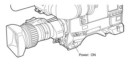
If condensation has occurred inside the unit, the HUMID display lights. In these cases, wait until the display goes off before proceeding to step 2.
